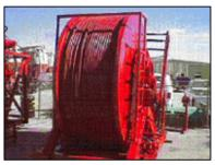
The tube comprises of thermoplastic liner at inner surface over-wound with a structural thermosetting laminate. Flexible tubing can be classified into two categories viz. bonded & unbonded type. In case of bonded coil tube, the thermoplastic liner and structural laminates are bonded together as one unit. On the other hand, unbonded tubing has flexibility to have a relative movement between each other. Unlike steel coil tubes, composite tubes are effective
